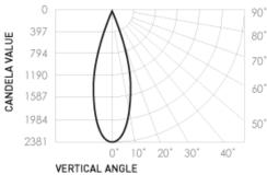
Source lumen output: 1255lm Delivered lumen: 815lm Efficacy: 49lm/W Colour temp.: 1.8K-3.1K (Night Shift) Beam angle: 38 (Special Order)° CRI: 97
