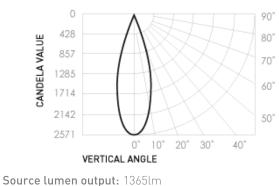
Delivered lumen: 880lm Efficacy: 53lm/W Colour temp.: 2700K (Special Order) Beam angle: 38 (Special Order)° CRI: 97
