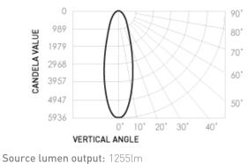
Delivered lumen: 815lm Efficacy: 49lm/W Colour temp.: 1.8K-3.1K (Night Shift) Beam angle: 24 (Special Order)° CRI: 97
