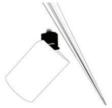
**Step 1** Align the track connector with the track.
